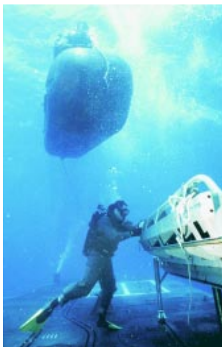
A Diver prepares the cradle to recover a SEAL Delivery Vehicle on the deck of an SSBN. The pilot of the SEAL Delivery Vehicle can be seen looking over the bow of the vehicle as he waits to make his approach. The track and cradle in the foreground is rolled out and back into the Dry Deck Shelter by the divers before and following each mission.
