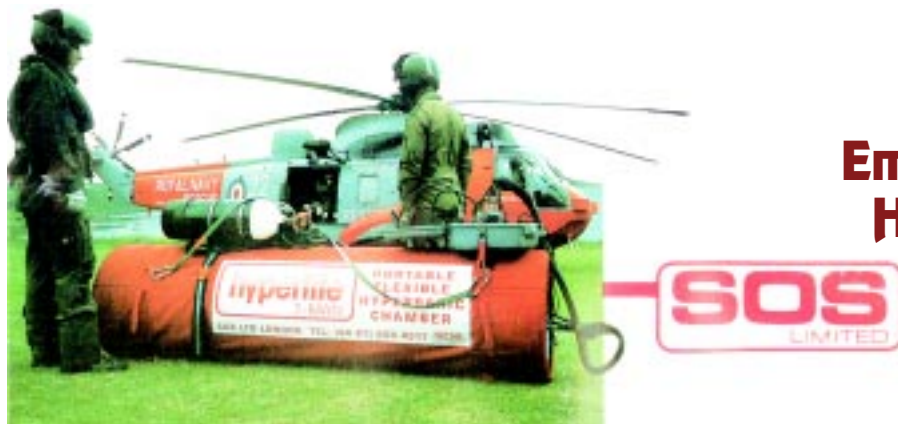
British Hyperlite (trademark) EEHS may provide a means of transporting a stricken diver while under treatment for Decompression Sickness
