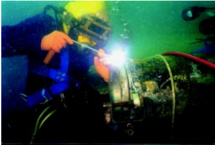
Welder/diver Scott Andersen welds the bellmouth on the towed array stowage tube. (Photo by BM1(DV) James Vaughan)
