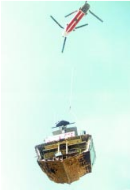
A section of the wheel house being air-lifted.
